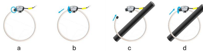
Figure 2-29 Rogowski Coil Installation Steps
